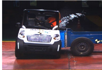
< Case 1, 4 : Release Belt, Separate Head & Torso >
