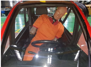
< Case 1, 4 : Release Belt, Separate Head & Torso >
