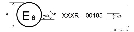
The above approval mark affixed to a vehicle shows that the type concerned was approved in Belgium (E6) pursuant to UN Regulation No. XXX. The first two digits (00) of the approval number indicate that the approval was granted in accordance with the requirements of UN Regulation No. XXX in its original form.
