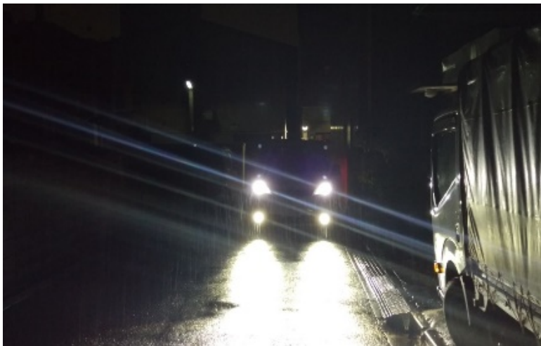
Fig.2 Reflective glare of headlights on a wet road
