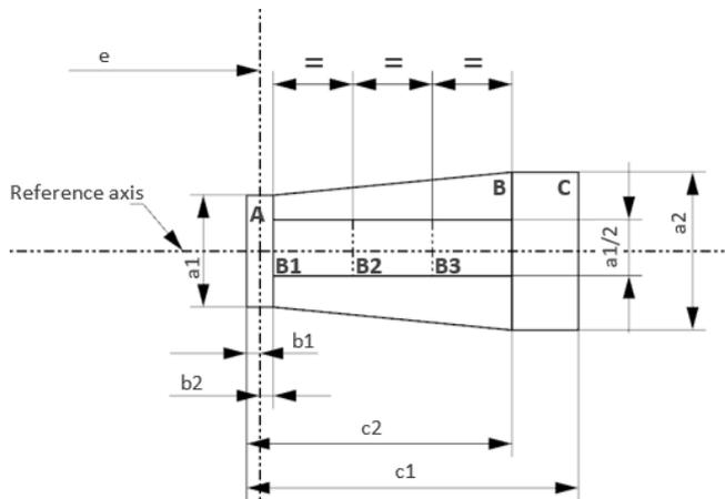
**Figure 8: Box specification of LED Replacement light source category, example H11/LED**
