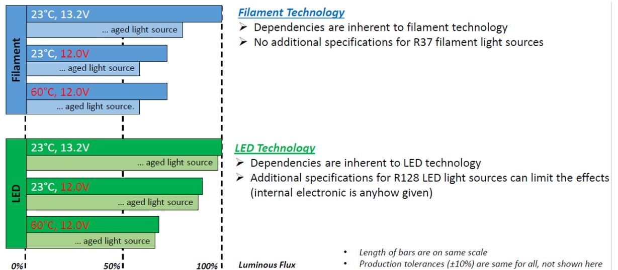
**Figure 10: Comparison of filament and LED technology with respect to the voltage- and temperature-dependency of the luminous flux (incl. ageing)**
