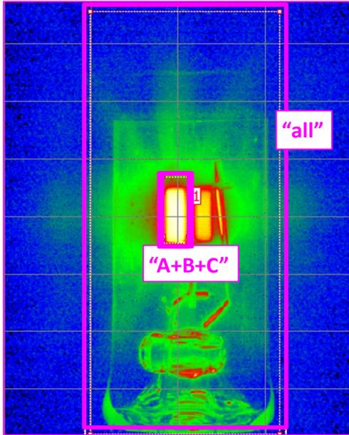
Figure 4: H11-sample showing typical situation of a filament light source with axial filament alignment
