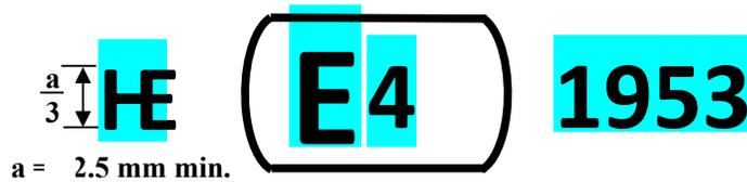
The approval mark above affixed to the light source, preceded by the character "HE", indicates a high-efficiency LED replacement light source that has been approved in The Netherlands (E 4) under the approval code 1953.
