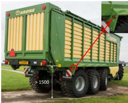
Figure 1 Position of additional reflectors: the lowest position of side reflectors are often above 1500 mm.
