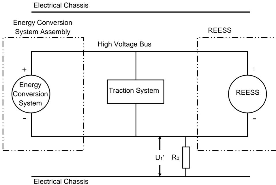
If  $U_2$  is greater than  $U_1$ , insert a standard known resistance ( $R_o$ ) between the positive side of the high voltage bus and the electrical chassis. With  $R_o$  installed, measure the voltage ( $U_2'$ ) between the positive side of the high voltage bus and the electrical chassis (see Figure 6 below). The electrical isolation ( $R_i$ ) is calculated according to the following formula:
