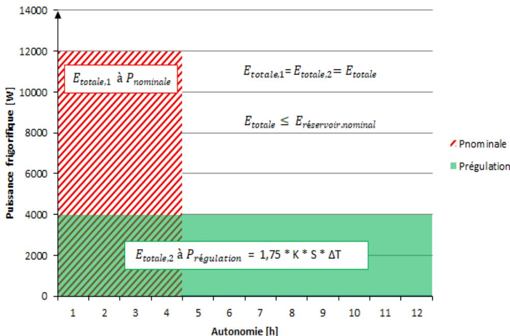
Negligible recharging time is deemed to be any operation lasting less than 20 minutes that allows for the recharging of the energy reservoir to its maximum starting with no more than one quarter of its nominal capacity.
