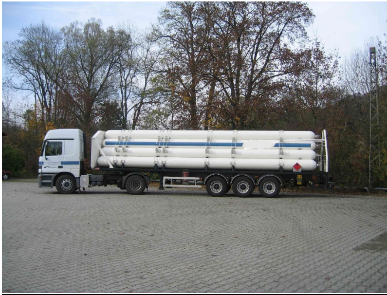
Battery vehicle constructed with seamless steel tubes
