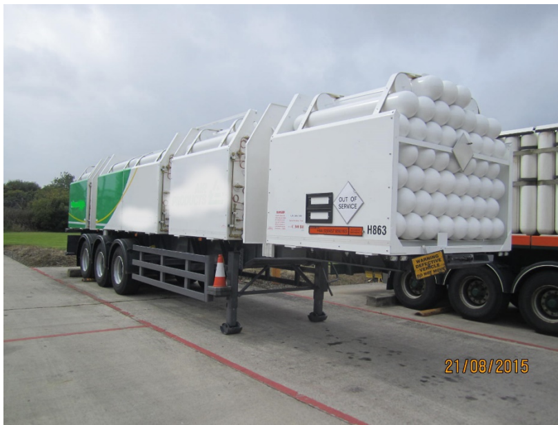
Battery vehicle constructed with seamless steel cylinders
