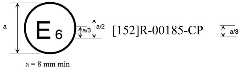
The above approval mark affixed to a vehicle shows that the vehicle type concerned has been approved in Belgium (E 6) with regard to the Advanced Emergency Braking Systems (AEBS) pursuant to Regulation No. [152] (marked with C for Car to Car, P for Car to Pedestrian). The first two digits of the approval number indicate that the approval was granted in accordance with the requirements of Regulation No. [152] in its original form.
