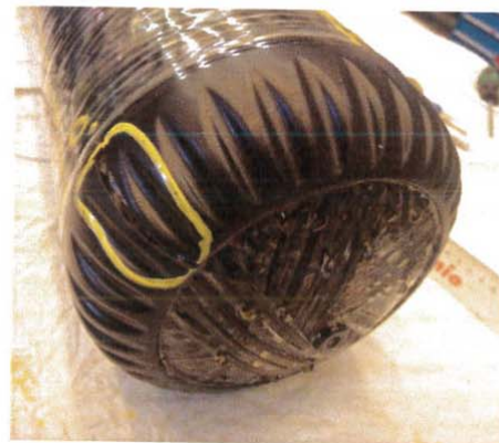
Figure 1-6: Damaged dome – Cylinder 6
