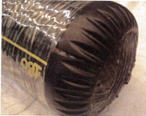
Figure 1-3: Damaged dome – Cylinder 1
