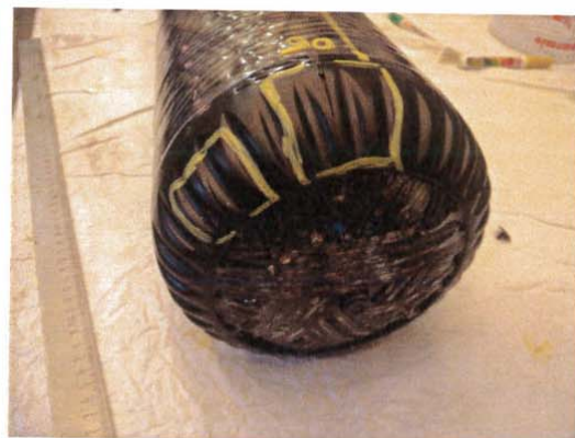
Figure 1-8: Damaged dome – Cylinder 11
