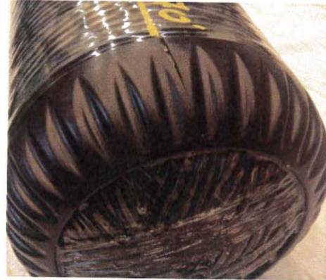
Figure 1-4: Damaged dome – Cylinder 2
