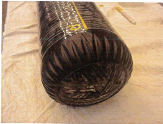
Figure 1-5: Damaged dome – Cylinder 5
