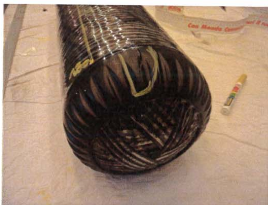
Figure 1-7: Damaged dome – Cylinder 10
