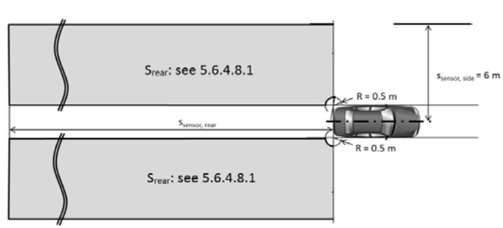
5.6.4.8.3. After each vehicle new engine start/run cycle (other than when performed automatically, e.g. the operation of a stop/start systems), the ACSF of Category [C1] function shall be prevented from performing a lane change manoeuvre until the system has detected, at least once, a moving object at a distance greater than [x] m.
