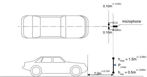
$\begin{array}{ll} \mathbf{h}_{\mathrm{min}} \colon & \mathrm{minimum\ height\ for\ measurements} \\ \mathbf{h}_{\mathrm{max}} \colon & \mathrm{maximum\ height\ for\ measurements} \\ \mathbf{P}_{\mathrm{I}\,\mathrm{max}} \colon & \mathrm{Point\ of\ maximum\ sound\ pressure\ level} \end{array}$
