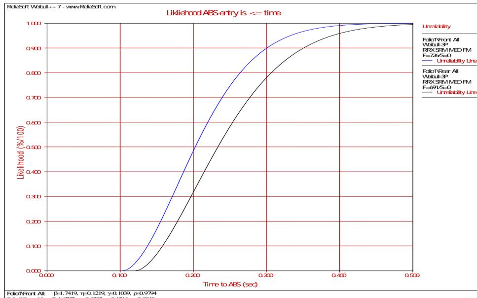
By reducing the lower limit to 0.1 seconds the test failure rate reduces to practically zero. Allowing the reduction tends to make the regulation more stringent by including a greater number of brake force application rates and eliminates restrictive test requirements.
