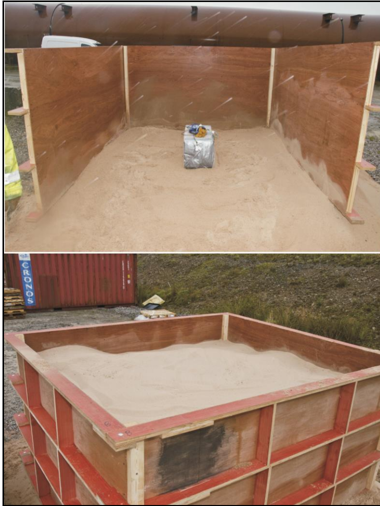
Figure 3: Method of burial of transport packs in wooden shuttering
