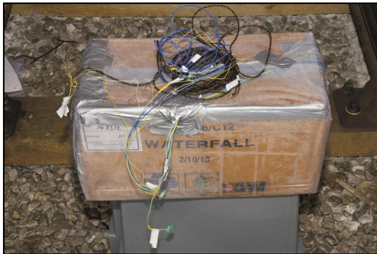
Figure 2: Method of sealing transport packs in plastic sheet
