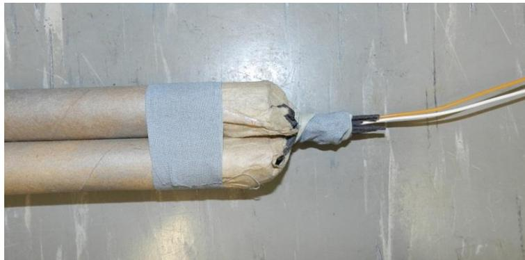
**Figure 7** – Method of igniting multiple articles, in this example two fountains
