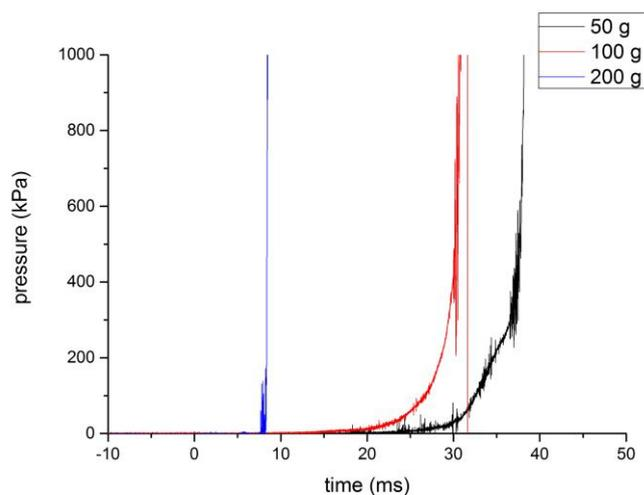
**Figure 4** – Time – pressure profile for burning of three amounts of waterfall composition.
