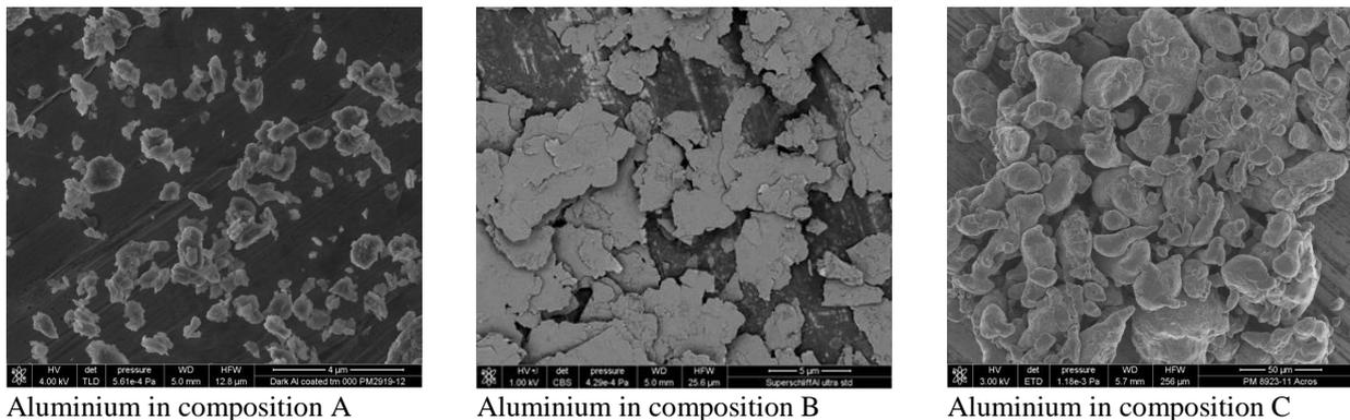
**Figure 9** – SEM photos of the 3 different types of aluminium, note the different scaling (4, 5 and 50 µm respectively)
