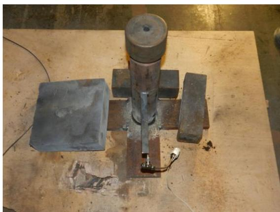
**Figure 2** – Impression of the test set-up with pressure transducer visible just below the steel blocks
