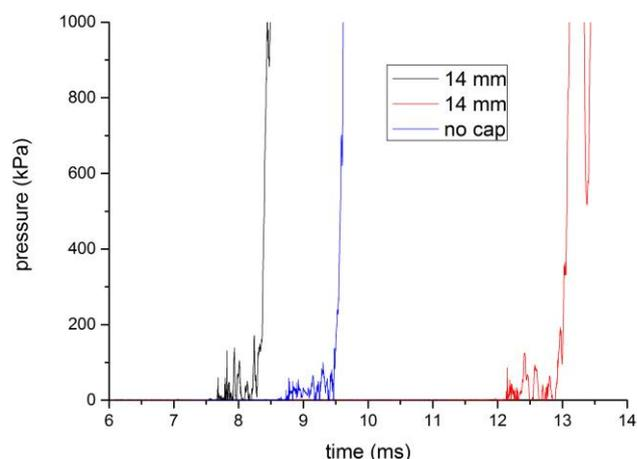
**Figure 5** – Time – pressure signal for burning 200 g waterfall composition with (black (same as in Figure 5) and red signal) and without the screw cap (blue signal).
