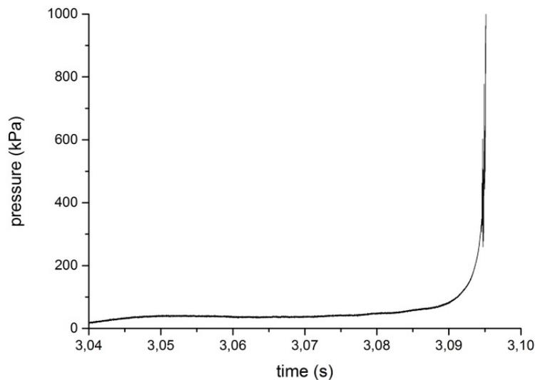
**Figure 6** – Time – pressure profile for burning of 100 g waterfall composition where ignition occurs on top of the pile
