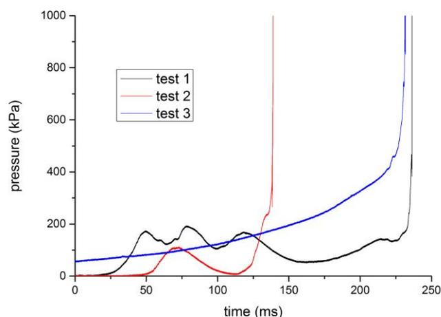
**Figure 8** – Pressure profile of three tests with three burning waterfall articles, showing an ‘instantaneous’ detonation (black and red signal) and regular burning before detonation occurred (blue signal, time shifted to fit).
