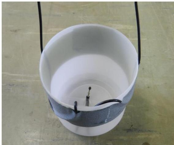
**Figure 3** – Plastics sample holder and electrical igniter for use in steel tube
