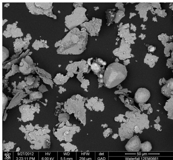
**Figure 1** SEM photo of the waterfall composition, the flake shaped particles are aluminium, the rounder particles are potassium perchlorate crystals, the dark particles are resin.
