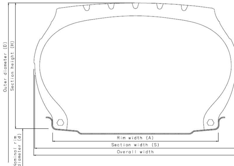
3.5.8. For other tyre sizes for which dimensions cannot be calculated, the dimensions including allowance for growth in service, shall comply with those given in standards publications of the organizations listed in Annex 10 and which were current either at the date of manufacture of the tyre or at any later date.
