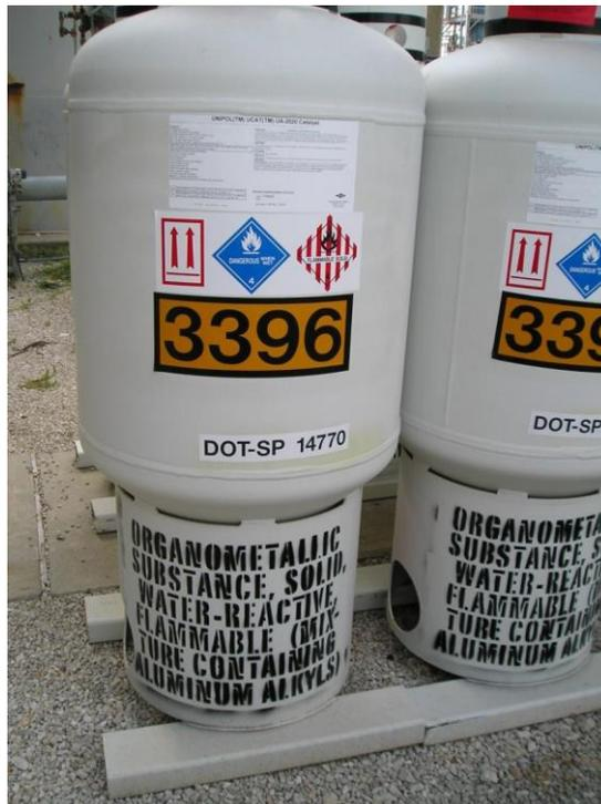
The label size (100 mm x 100 mm) is not in compliance with the placarding requirements (250 mm x 250 mm, four sides) of the Model Regulations, however are in compliance with CFR 49 §172.514 (c)(1); permitting labels as an alternative to placards.
