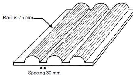
Dimension of the crush plate:
