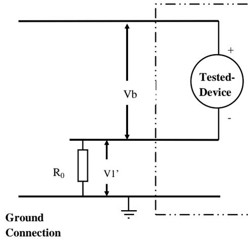
If V<sub>2</sub> is greater than V<sub>1</sub>, insert a standard known resistance (R<sub>0</sub>) between the positive pole of the Tested-Device and the ground connection. With R<sub>0</sub> installed, measure the voltage (V<sub>2</sub>\') between the positive pole of the Tested-Device and the ground connection (see Figure 3).
