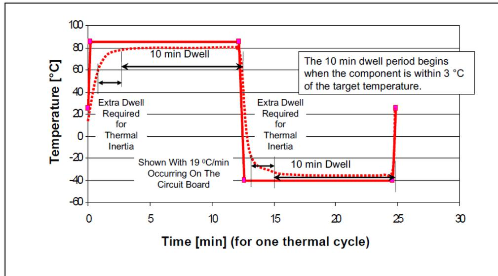
18. Since the REESS has a different thermal mass and has different operation and storage temperature ranges than typical electric / electronic components, a modification of the test conditions i.e. lower maximum temperature and longer dwell time are needed.
