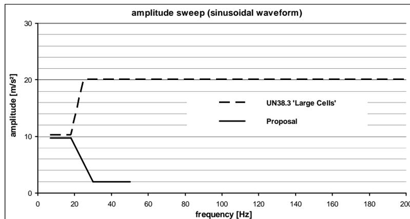
6. The test duration is also aligned with UN38.3, Test T3, requiring 12 transitions from the minimum to the maximum frequency and back within 15 min., resulting in a total test duration of 3 hours.
