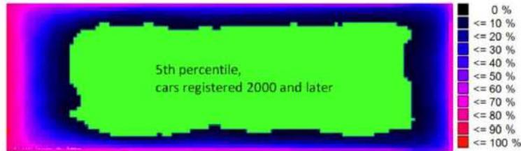
35. The dimension of the restricted mounting zones for the generically approved REESS is derived from the Japanese regulation Attachment 111 (technical standard for protection of occupants against high voltage after collision in electric vehicles and hybrid electric vehicles).
