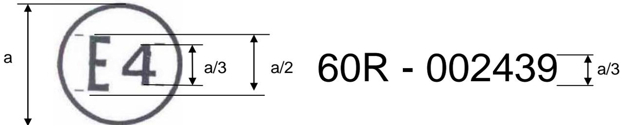
The above approval mark affixed to a vehicle shows that the vehicle type concerned has, with regard to the driver-operated controls, been approved in the Netherlands (E 4) pursuant to Regulation No. 60 under approval number 002439. The approval number indicates that the approval was granted in accordance with the requirements of Regulation No. 60 in its original form.
