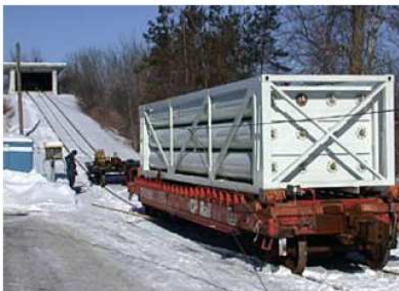
Figure 2: MEGC undergoing an impact test
