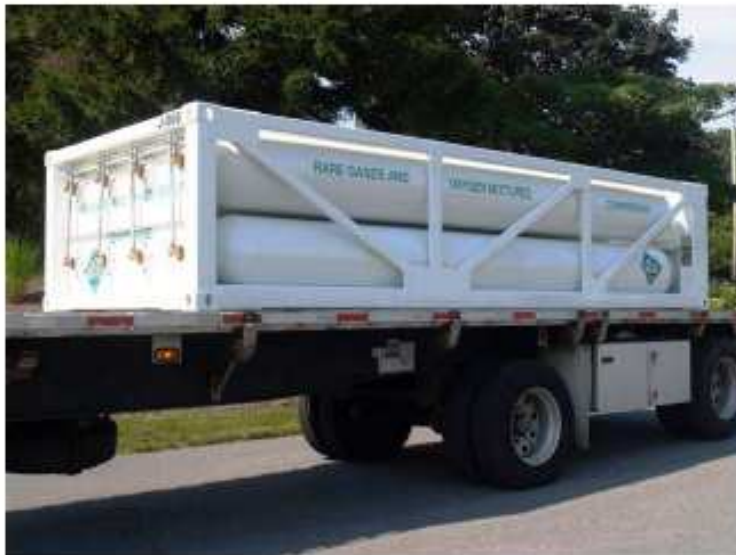
Figure 6: 20-foot-long MEGC (half-length and half-height – 8 tubes)
