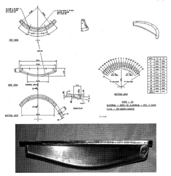
Figure 4 Type 2C Bead Unseating Block and Adaptor
