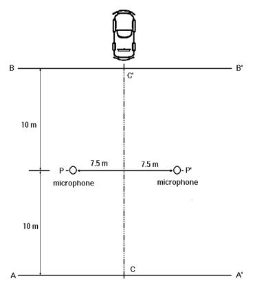
Figure 1. Microphone positions for the measurement
