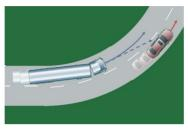
6.5.7.1. The subject vehicle shall approach and pass the target vehicle at a closing speed of 10 km/h when both vehicles are travelling in the centre of adjacent lanes, each 3.5m wide, with the inner marking of the inside lane having a 125m radius of curvature. The target vehicle shall travel at a constant speed of 40 km/h.
