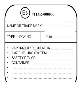
The above plate, with approval mark and some technical information on the retrofit system, has to be fixed permanently on the body of the vehicle.
