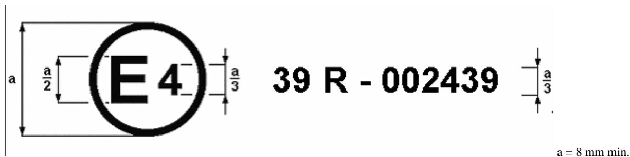
The above approval mark affixed to a vehicle shows that the vehicle type concerned has, with regard to the equipment of temporary-use spare unit(s), been approved in the Netherlands (E 4), pursuant to Regulation No. 64 under approval number 012439. The approval number indicates that the approval was granted in accordance with the requirements of Regulation No. 64, incorporating the 01 series of amendments.
