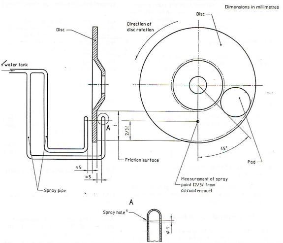
a. Disc Brakes : Sketch of water spray equipment:
