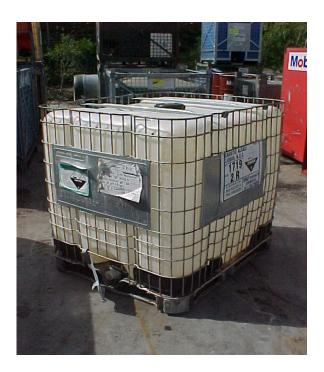
Lightweight IBC: designed with minimum outer packaging, particularly on the upper surface, and specially designed pallet base. The inner plastic receptacle of this unit has bulged out under load and has deformed the outer metal receptacle.
