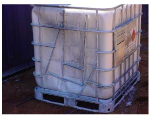
The damaged IBCs after being removed. The IBC on the left has suffered a complete structural failure of the outer casing and the "rigid" inner receptacle has been forced out. The IBC on the right has failed due to the pressure applied to the outer casing by the bulging inner receptacle of the other IBC. Again there is no damage to the leading corners of either IBC that would indicate a significant impact during loading operations.
