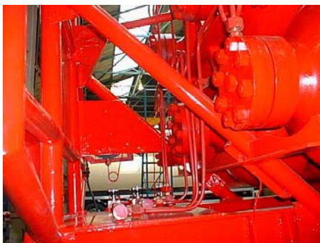
Fig. 4a) Tubes with stop valves mounted on vehicle chassis
