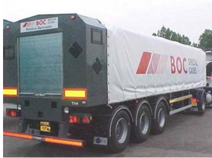
Fig. 5a) Battery-vehicle with tubes
