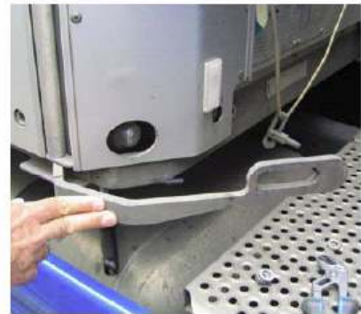
Inner side of the chassis frame – the lock tab nut is NOT secured.
