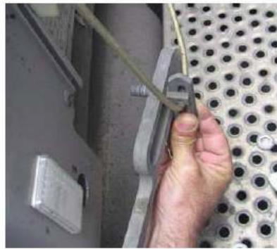
Inner side of the chassis frame – the lock tab nut is NOT secured.
