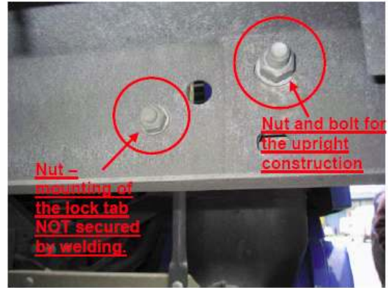
Inner side of the chassis frame – the lock tab nut is NOT secured.
