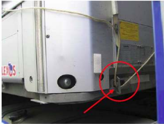
Lock tab secured by the TIR wire.
