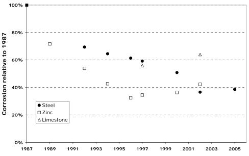
Figure 1. Average trends in corrosion relative to the first exposure in 1987.
