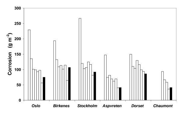
Figure 2. Trends in carbon steel corrosion showing values for the periods 1987/1988, 1992/1993, 1994/1995, 1997/1997, 1997/1998, 2000/2001, 2002/2003 and 2005/2006 (the last is marked in black). The Chaumont site was not part of the original network and monitoring started in 1996.
