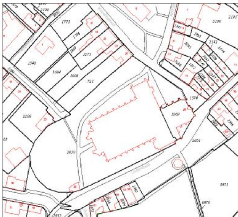
Figure X. Extract from an urban cadastral plan (thick lines) with topographic data (thin lines with red for buildings in the Netherlands)
