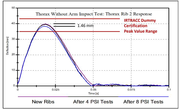
Theoretical IRTRACC responses obtained from WorldSID 50<sup>th</sup> percentile adult male dummy with RibEye towards the middle of the ISO 15830 certification corridor for WorldSID with IRTRACC.
