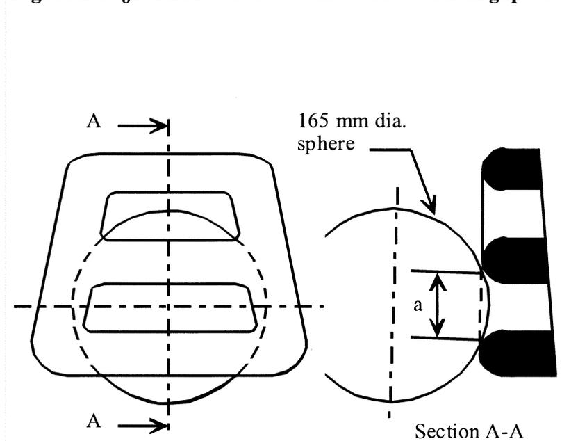
Figure 3 of §571.202a - Measurement of a horizontal gap "a".
