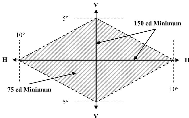
If visual examination of a light appears to reveal substantial local variations of intensity, a check shall be made to ensure that, outside the axes, no intensity
