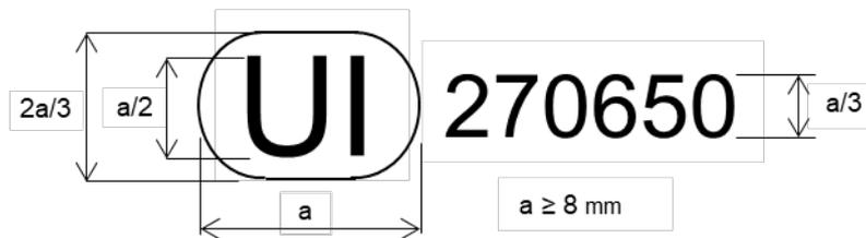
The above Unique Identifier marked on the lamp shows that the type concerned has been approved and that the relevant information on that type approval can be accessed on the UN secure internet database by using 270650 as the Unique Identifier.
