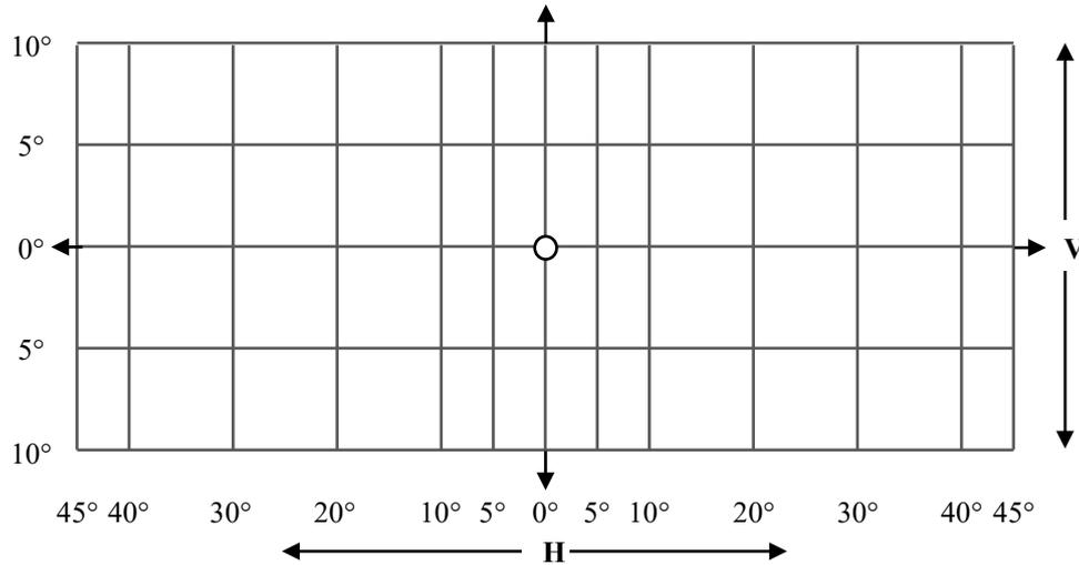
Minimum values: 0.6 cd at any point other than the reference axis, at which it shall be 4.0 cd
