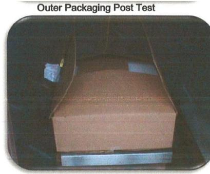
15. Prior to the test, the package had been opened to place the thermocouples into the middle of the material. In spite of this weakening effect, no product could escape, as it was fully polymerized. The package was not damaged by the heat that developed during the test. Therefore, the criteria that are proposed are fulfilled:
