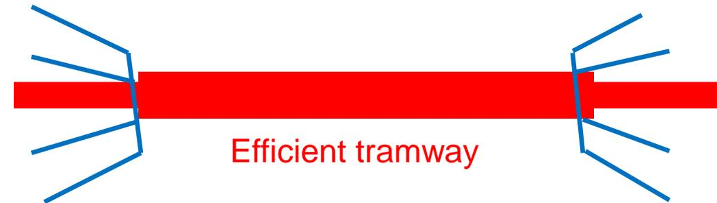
Efficiency of large capacity vehicles can be achieved only by means of passenger flow concentration on trunk routes, with removal of duplicate routes.
