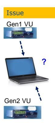
It is not easy for data analysis tools to distinguish between data downloaded from a Gen1 VU memory and data downloaded from a Gen2 VU memory. This is because data identifiers used in the download protocol are the same.
