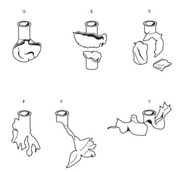
Figure 2. Tube deformation, fragmentation patterns and effect levels reproduced from Figure 18.6.1.3 of MTC6.
