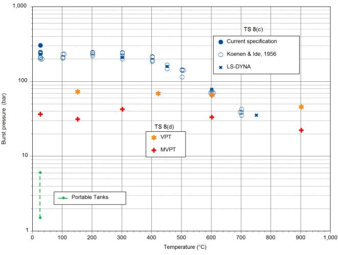
burst pressure specified for T1/T2 Portable Tanks, the range of which extends from 1.5bar to 6 bar.
