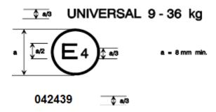
The child restraint system bearing the above approval mark is a device capable ...
