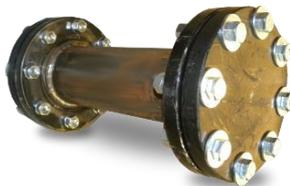
13. Testing was performed on the DOT-SP 13481, 3rd Revision, shipping container to verify that ignition of 25 grams of liquid does not result in breaching or fragmenting the pipe. 25 grams of nitroglycerin was placed inside the pipe with a blasting cap. No hazardous effects were observed outside the shipping container: the pipe was not breached or cracked or fragmented. Below is an image of the post-test result.
