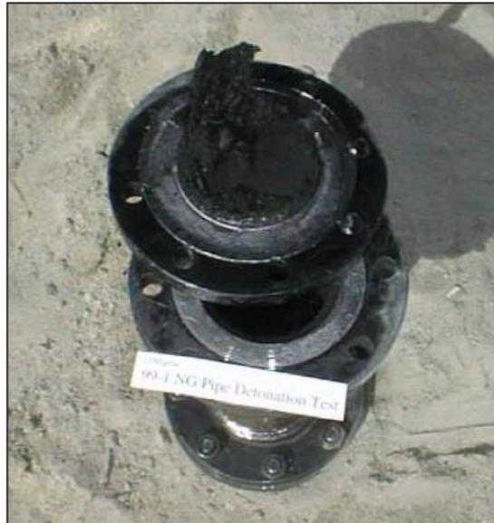
14. A bonfire test was also completed where 25 grams of PETN was placed inside the pipe. Below is a picture showing the pipe following the test. No hazardous effects were observed outside the shipping container.
