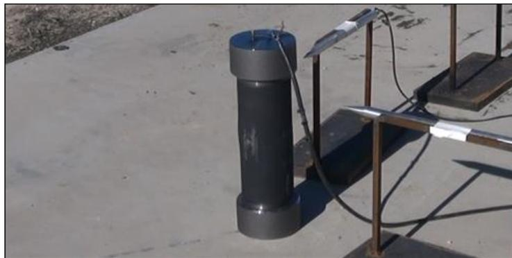
9. An external fire test was also completed to verify that the 25 grams of dry PETN does not result in fragmentation or damage to the pipe. Below is a picture showing the pipe following the test.
