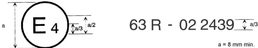
The above approval mark affixed to a vehicle shows that the vehicle type concerned has, with regard to its ~~noise~~ **sound** emission, been approved in the Netherlands (E 4) pursuant to Regulation No. 63 under approval No. 022439. The approval number indicates that the approval was granted according to the requirements of Regulation No. 63 as amended by the 02 series of amendments.
