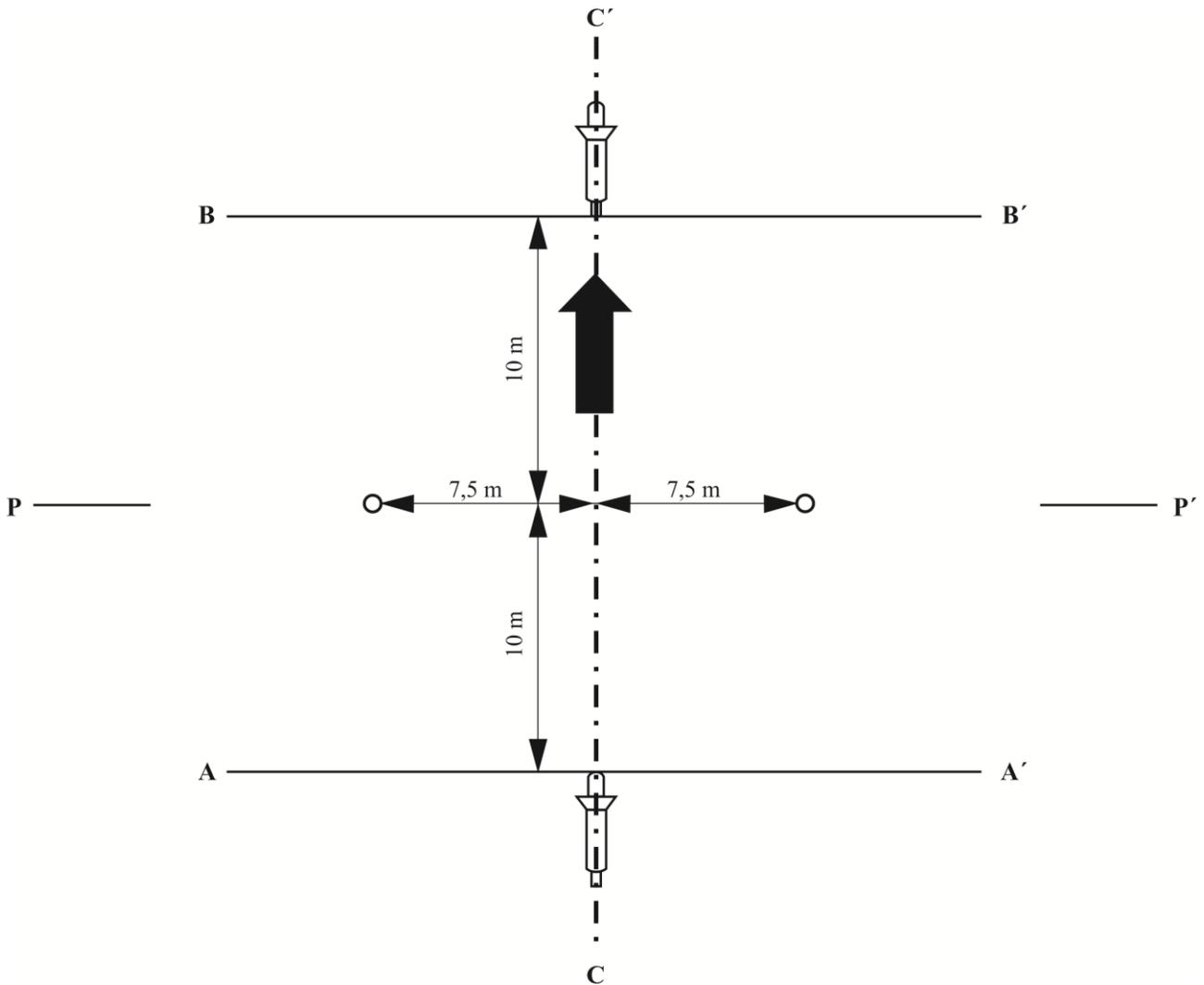
**Two lines, AA' and BB', parallel to the microphone line PP' and situated respectively 10 m forward and 10 m rearward of that line shall be marked out on the test track.**
