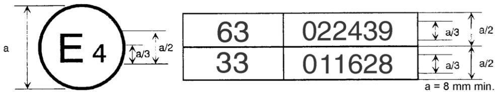
The above approval mark affixed to a vehicle shows that the vehicle type concerned has been approved in the Netherlands (E 4) pursuant to Regulation Nos. 63 and 33.<sup>1</sup> The approval numbers indicate that, at the dates when the respective approvals were given, Regulation No. 63 included the 02 series of amendments and Regulation No. 33 has also been amended by the 01 series of amendments.
