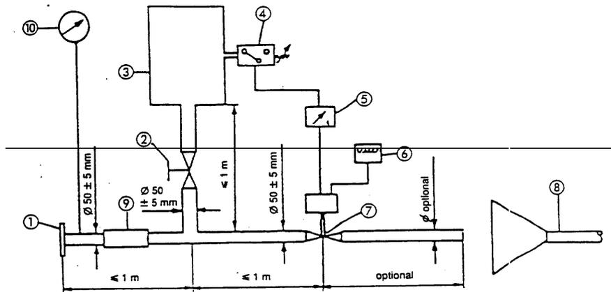
**Test apparatus for conditioning by pulsation**
