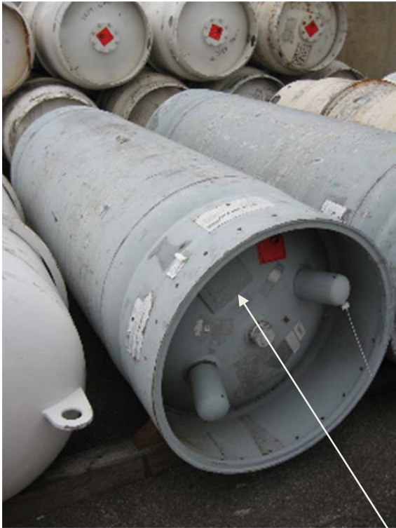
Example of location of pressure drum nameplate
