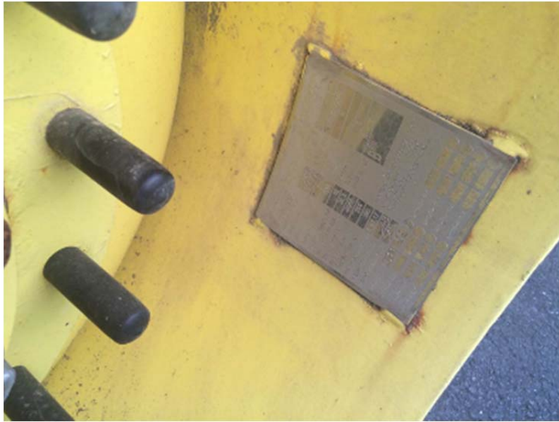
Example of location of a nameplate on the inner face of the pressure drum shroud
