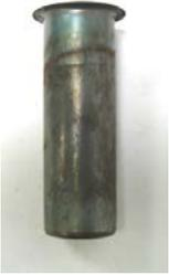
**“A”:** Bottom of the tube bulged out
