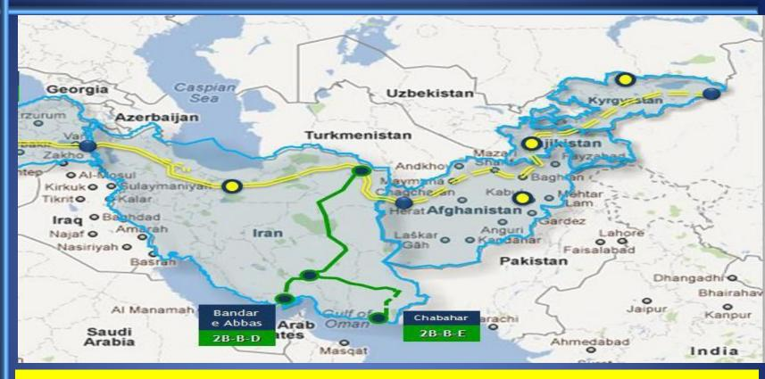
The Project of construction of railway from China to Europe through Kyrgyz Republic-Tajikistan-Afghanistan -Iran (KTAI) is coordinated by ECO. The total length of the (Kashghar-Herat) route is around 2155 km. The total length of Sangan (Iran)-Herat Railway line is 191 km out of which 76 kilometers lying in Iranian territory has already been constructed.
