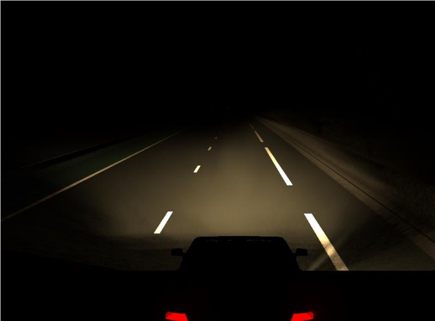
Figure 3. Visual aspect of a low beam producing 140 Lumen in Zone I
