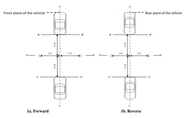
Figure 2a and 2b Measuring positions for vehicles in motion in-door and in stationary
