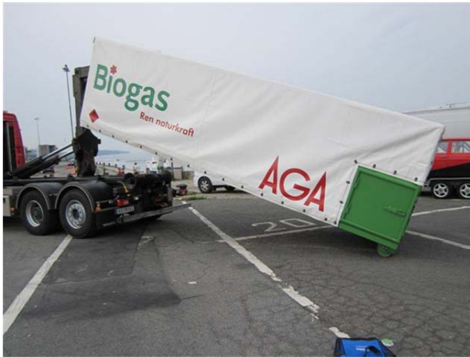
A MEGC being unloaded from a truck by the hooklift hoist
