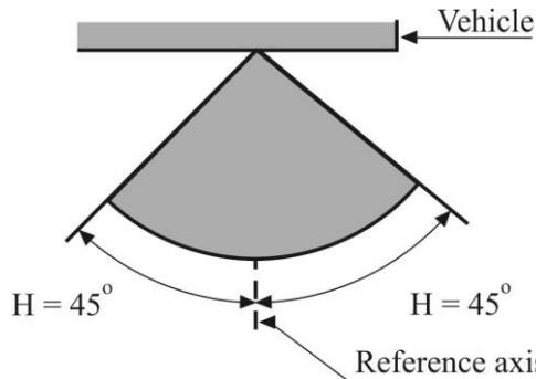
However, in the case of a pair of lamps, the inboard geometric visibility requirement is deemed to be satisfied if the lamps conform to the photometric values prescribed in the field of light distribution for the approval of the device.
