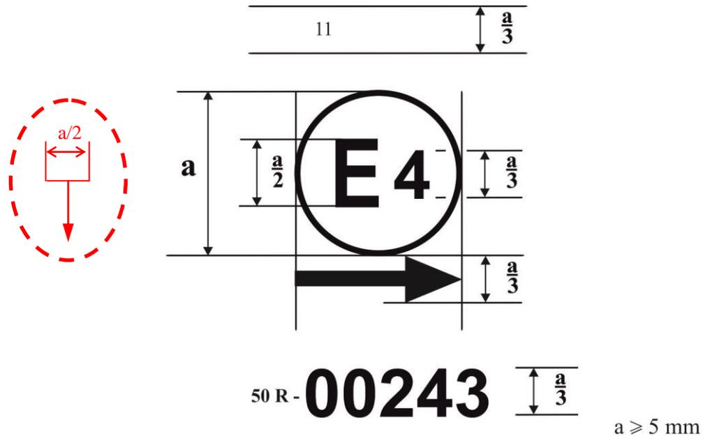
A device bearing the approval mark shown above is a direction indicator of the category 11 approved in the Netherlands (E4) under the number 00243. The first two digits of the approval number indicate that the approval was granted in accordance with the requirements of Regulation No. 50 in its original form.
