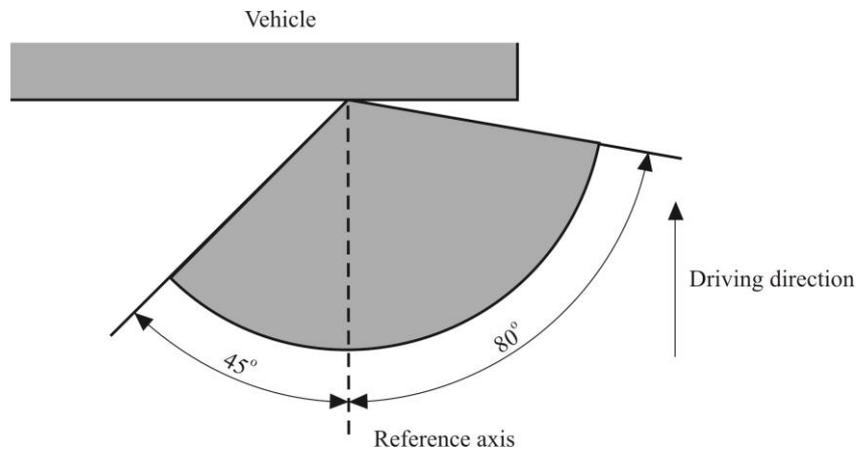
**However, in the case where a device is intended to be installed with its H plane at a mounting height less than 750 mm above the ground, the inward angle of 45° may be reduced to 20° under the H plane."**
