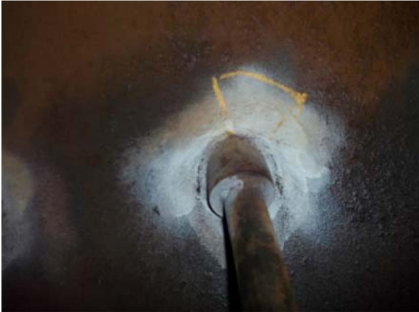
Nozzle 2 is the tanker filling connection (is connected to internal fill pipework) and has a 90 mm long crack as indicated below:
