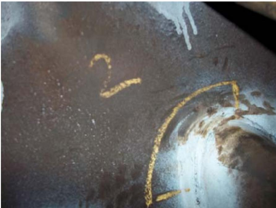
Nozzle 3 is the tanker vapour balance connection (and again is connected to internal pipework) and has a 50 mm long crack as indicated below:
