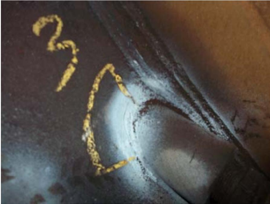
The magnetic particle examination of a weld (undertaken in 1995 as part of a companies procedure when it purchasing a used fixed tank, that was constructed in 1973 by a very reputable tank manufacturer) around part of the main outlet connection nozzle identified that the internal root weld was missing and it just had a cap weld.
