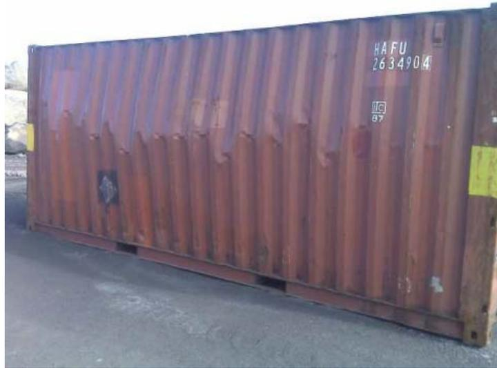
Figure 1: Closed container damaged due to pressure build-up with dross residue.
